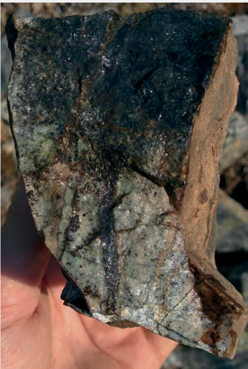
Above: QSP altered porphyry with quartz sulfide veins. Left : Hornfels with patchy/vein biotite magnetite sulfides. Below : Intense stockwork to sheeted quartz sulfide veining in trench.
