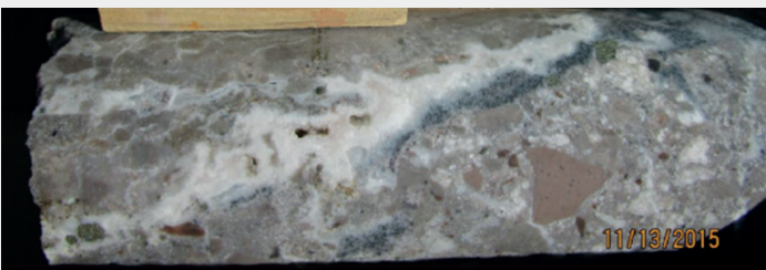
Core from drill hole TMD-15-05 at approximately 275.5 m: Hydrothermal breccia with polymictic fragments, mostly sub-rounded and less angular, comprising siltstone and sandstone in a dolomitic matrix, from an interval grading 0.79% Zn, 107 ppm Pb, 29 ppm Cu and 1.45 g/t Ag (Candia and Oviedo, 2016).
