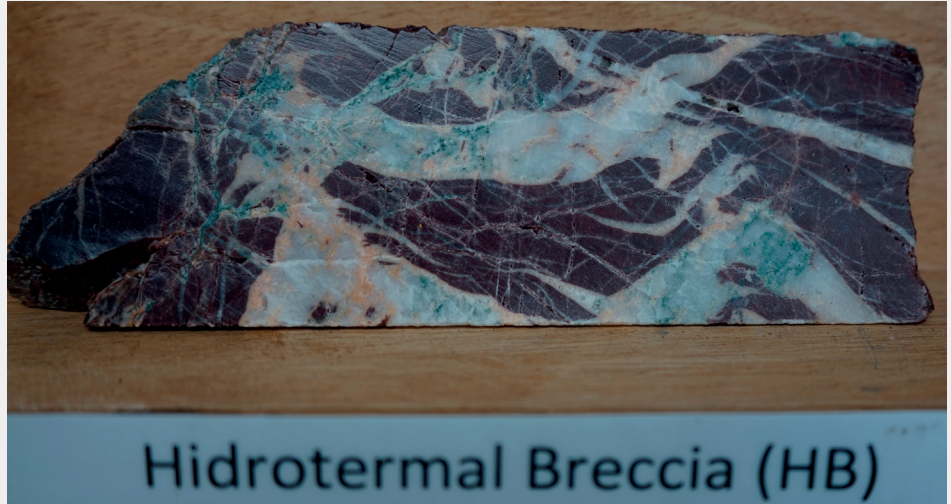
Core displaying the volcanoclastic breccia unit at Infanta. This breccia is the rock type most commonly found immediately above the mineralized horizon.
