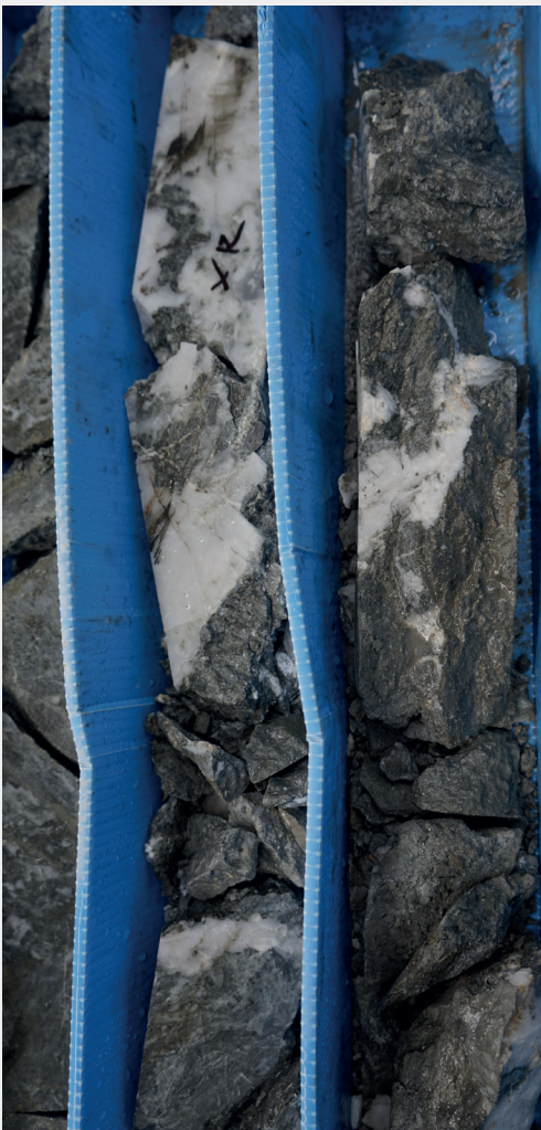
Stockwork mineralization with intense quartz veining in core from Infanta.
