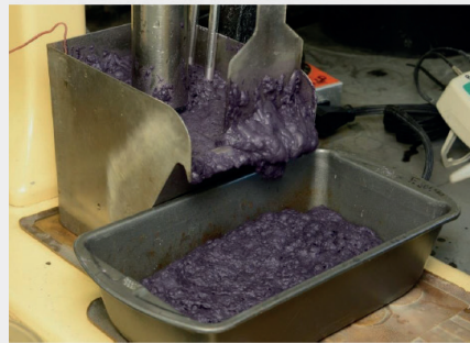
Flotation test to produce acid-spar concentrate
