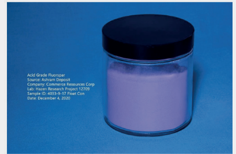
0.5 kg sample of >98% CaF 2 acid-spar delivered to global commodities trader
