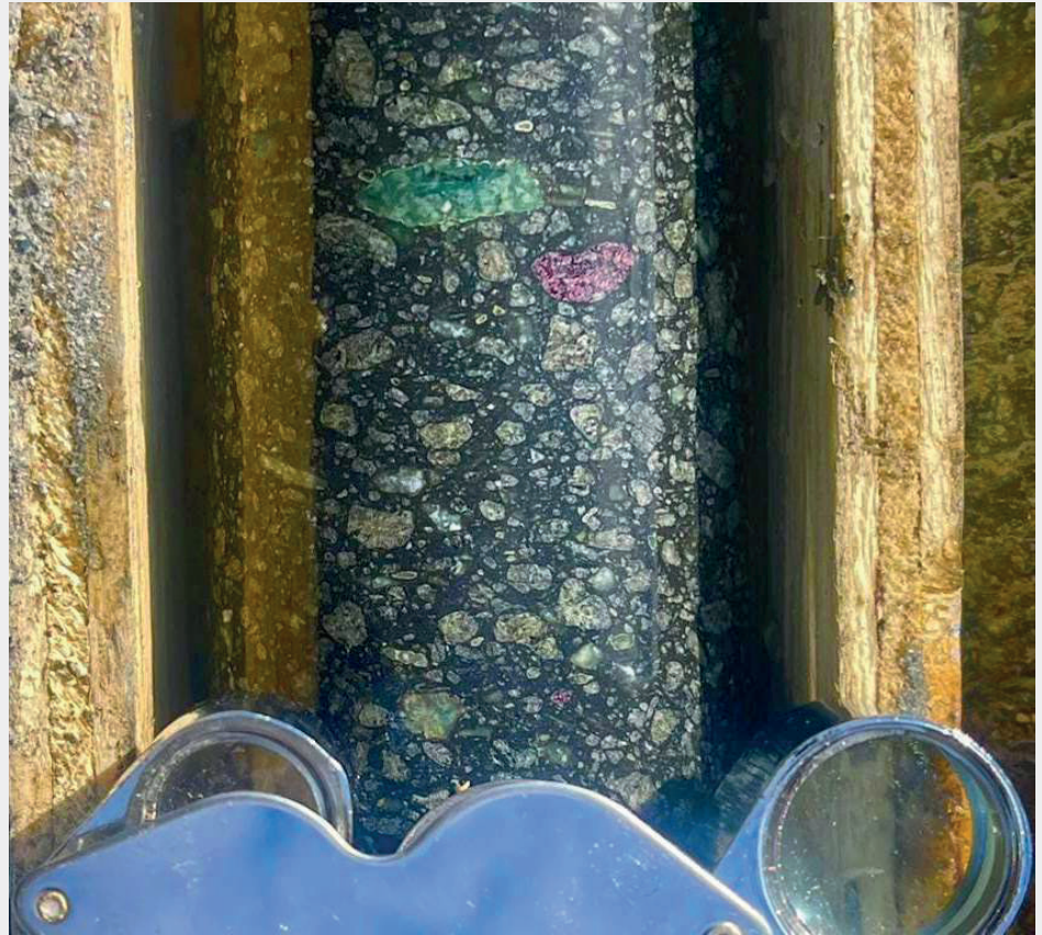
Drill core from the Arbutus Kimberlite with chrome diopside (green) and garnet (burgundy red) as prominent indicator minerals, along with abundant coarse olivine in a dark matrix. ( Source )
