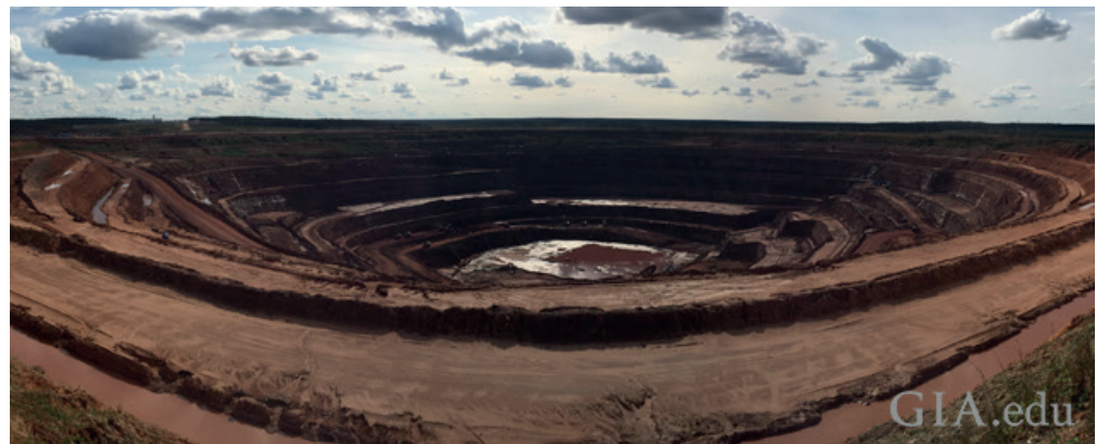
The open-pit of Alrosa's Arkhangelskaya Kimberlite Pipe . This was the first kimberlite to be developed at Lomonosov because it had the highest diamond grade and the least overburden. (Photo by Karen Smit/GIA , 2016)
